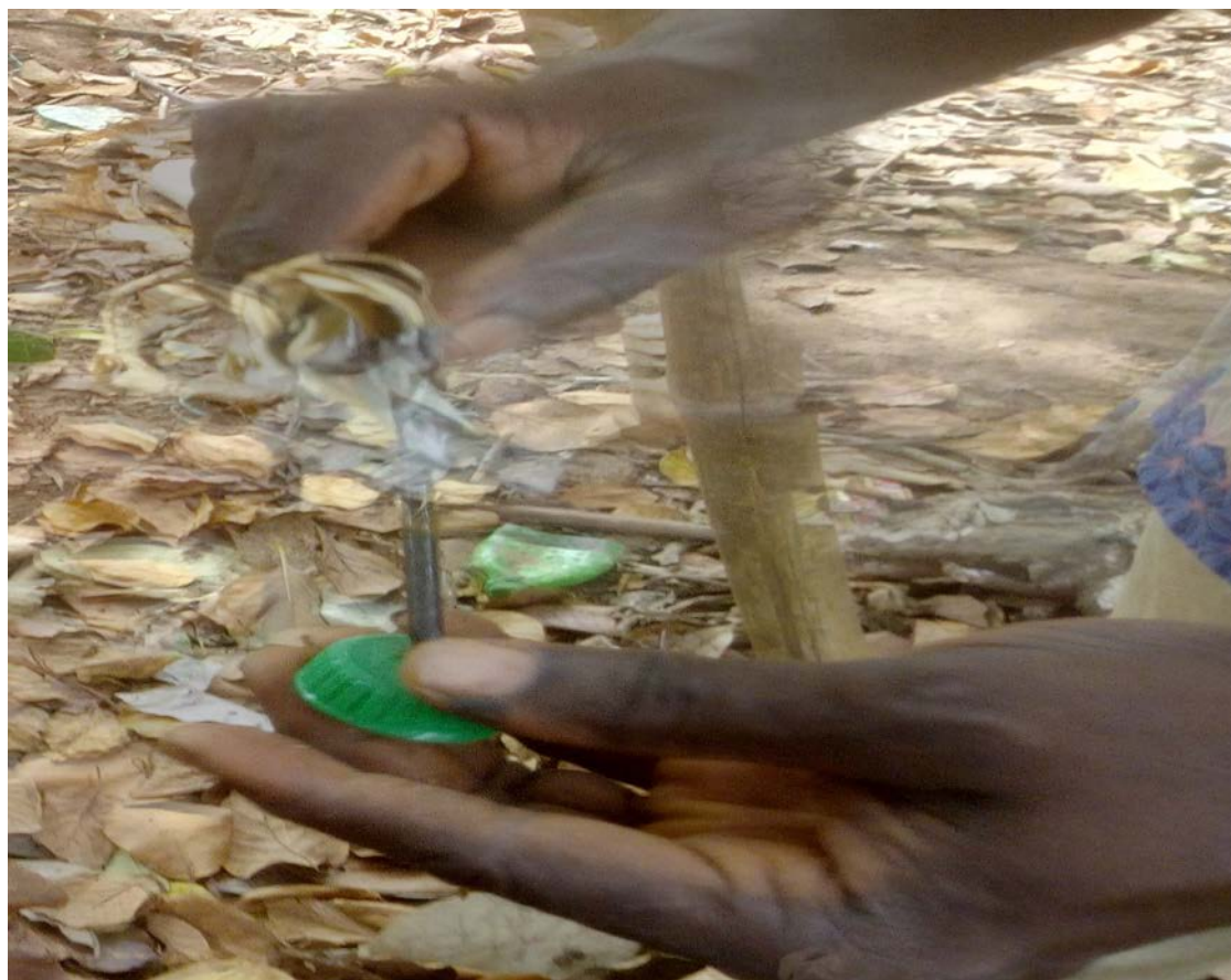
PLATE.13, USING HOT NAIL TO BORE HOLE IN WASTE WATER CAN COVER FOR EFFLUENT STORAGE
