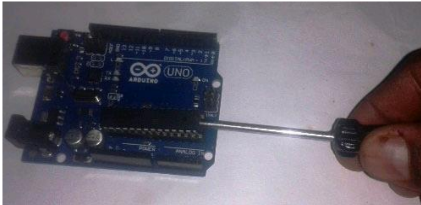
Figure 5: An Arduino IC being removed from the Arduino board
