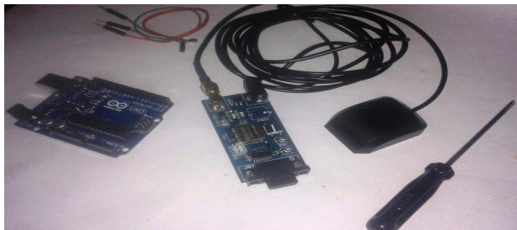
Figure 4: Arduino Use in Interfacing a GPS
