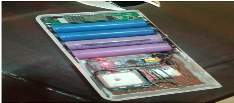
Figure 5: GSM Based Anti-Theft Vehicle Security System
